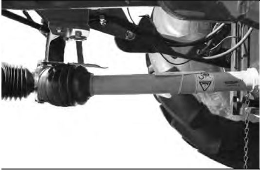
Fig. 28 PTO shaft connections at the same height
