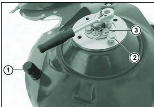
Fig. 63 Tightening the inner bolts
