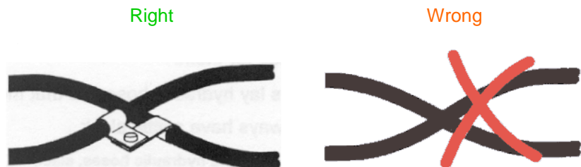
Fig. 4: Laying hydraulic hoses, crossing
